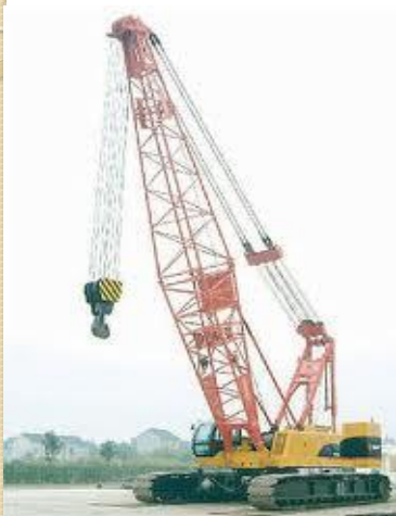
Crawler Mounted Crane
